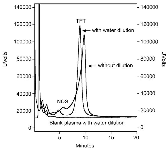
Fig. 3. Chromatograms of plasma TPT/NDS (50/5.0 ng/mL) with and without water dilution compared to blank plasma with water dilution. The same HPLC conditions as described in Fig. 2.
