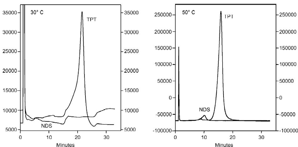
Fig. 2. Chromatograms for (A) TPT (100 ng/mL) and NDS (10 ng/mL) at 30 °C and (B) at 50 °C. HPLC conditions: Zorbax SB-C<sub>18</sub> (75×4.6, 3.5 μm) with Varian Guard column (10×3 mm); 22% MeOH with 75 mM KH<sub>2</sub>PO<sub>3</sub> + 0.2% TEM and flow-rate 1.0 mL/min.
