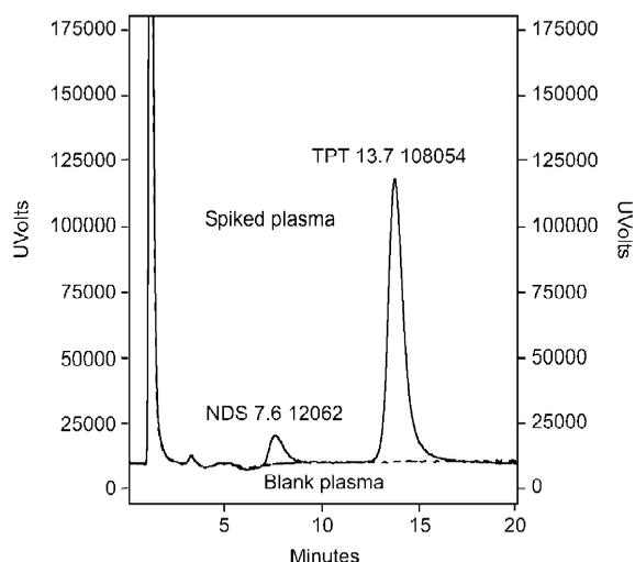
Fig. 5. Chromatogram overlays for plasma TPT/NDS (50/5.0 ng/mL) and blank plasma at optimized HPLC conditions: Zorbax SB-C<sub>18</sub> (150×3.0, 3.5 μm) with Varian Guard column (10×3 mm); 27% MeOH with 75 mM KH<sub>2</sub>PO<sub>3</sub>+0.2% TEM at pH 6.5 and flow-rate 0.8 mL/min.
